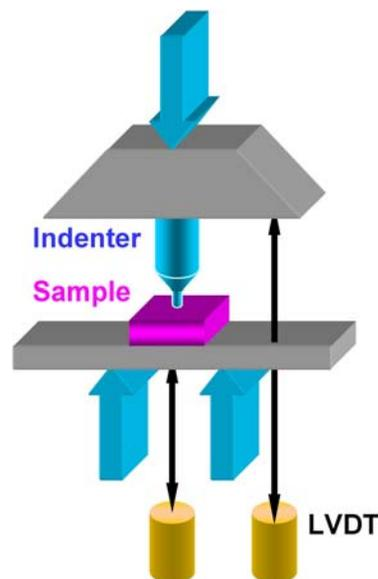
Fig. 1. Schematic illustration of the impression creep test.
