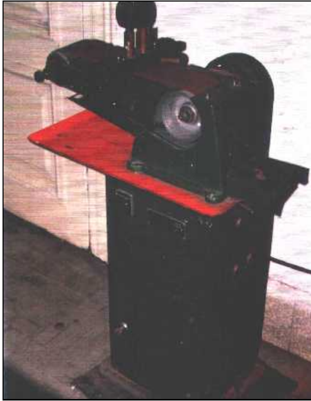
Fig. 2. The pin-abrasion testing machine.
