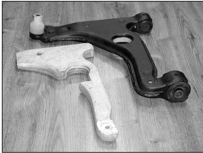
Fig. 8. Complex welded part with AlSi12 aluminium foam insert.
