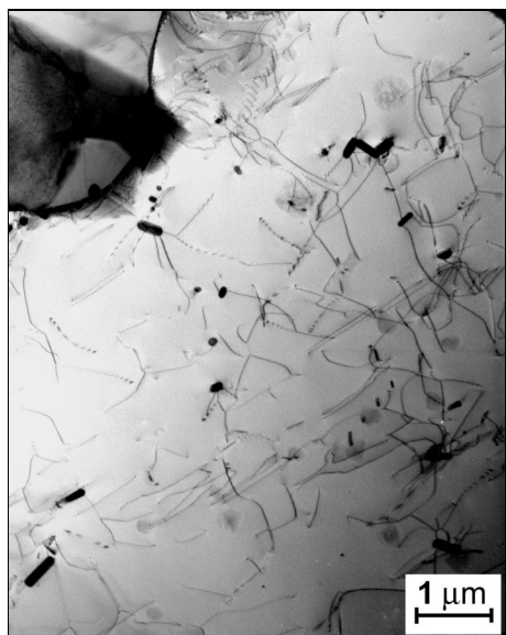
Fig. 5. Microstructure after creep at 600°C of the material annealed before deformation at 1150°C/2 h.
