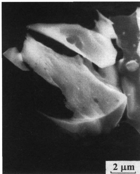
Fig. 3. Ion thinned NiCrAlY powder with a spherical cap (SEM).
