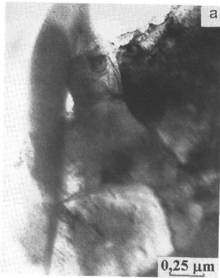
Fig. 7a. Microstructure of NiCrAlY metal-oxide interface (TEM, BF image).
