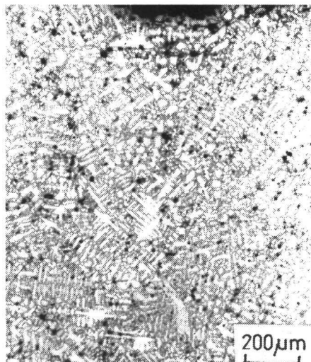
Fig. 3. As cast, not deformed microstructure of the cutting edge of the sickle P-6426.
