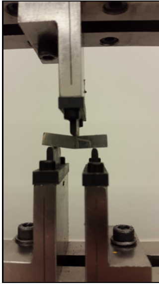
Fig. 1. The three-point bending testing of the composite sample.
