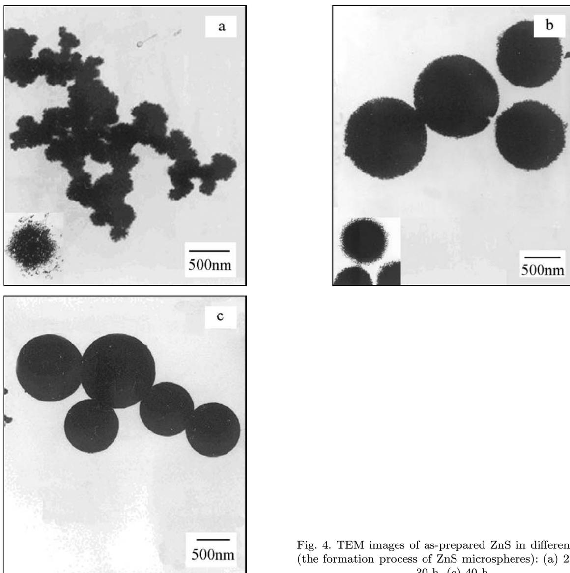
Fig. 4. TEM images of as-prepared ZnS in different stages (the formation process of ZnS microspheres): (a) 25 h, (b) 30 h, (c) 40 h.
