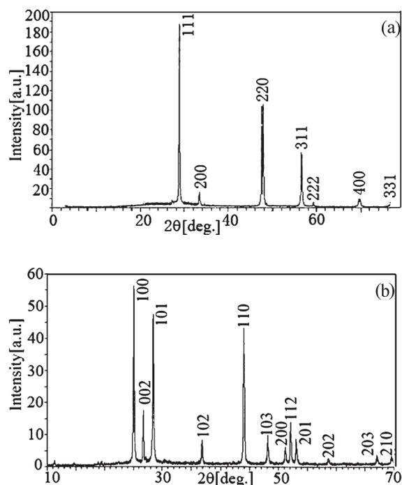
Fig. 2. XRD patterns of ZnS (a) and CdS (b) nanoparticles assemblies.
