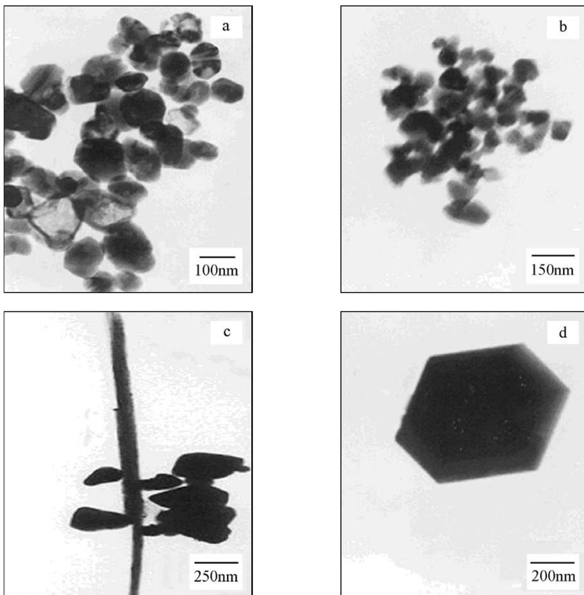
Fig. 5. TEM images of ZnS (a) and CdS (b) prepared without template; ZnS (c) and CdS (d) using 8-hydroxyquinoline as template.
