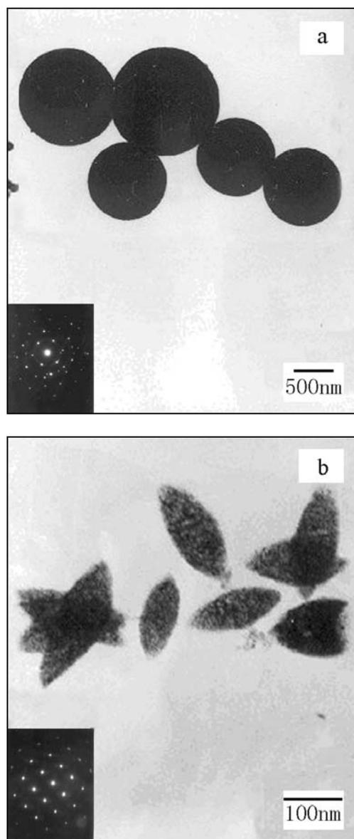
Fig. 1. TEM images of ZnS (a) and CdS (b) as prepared.
