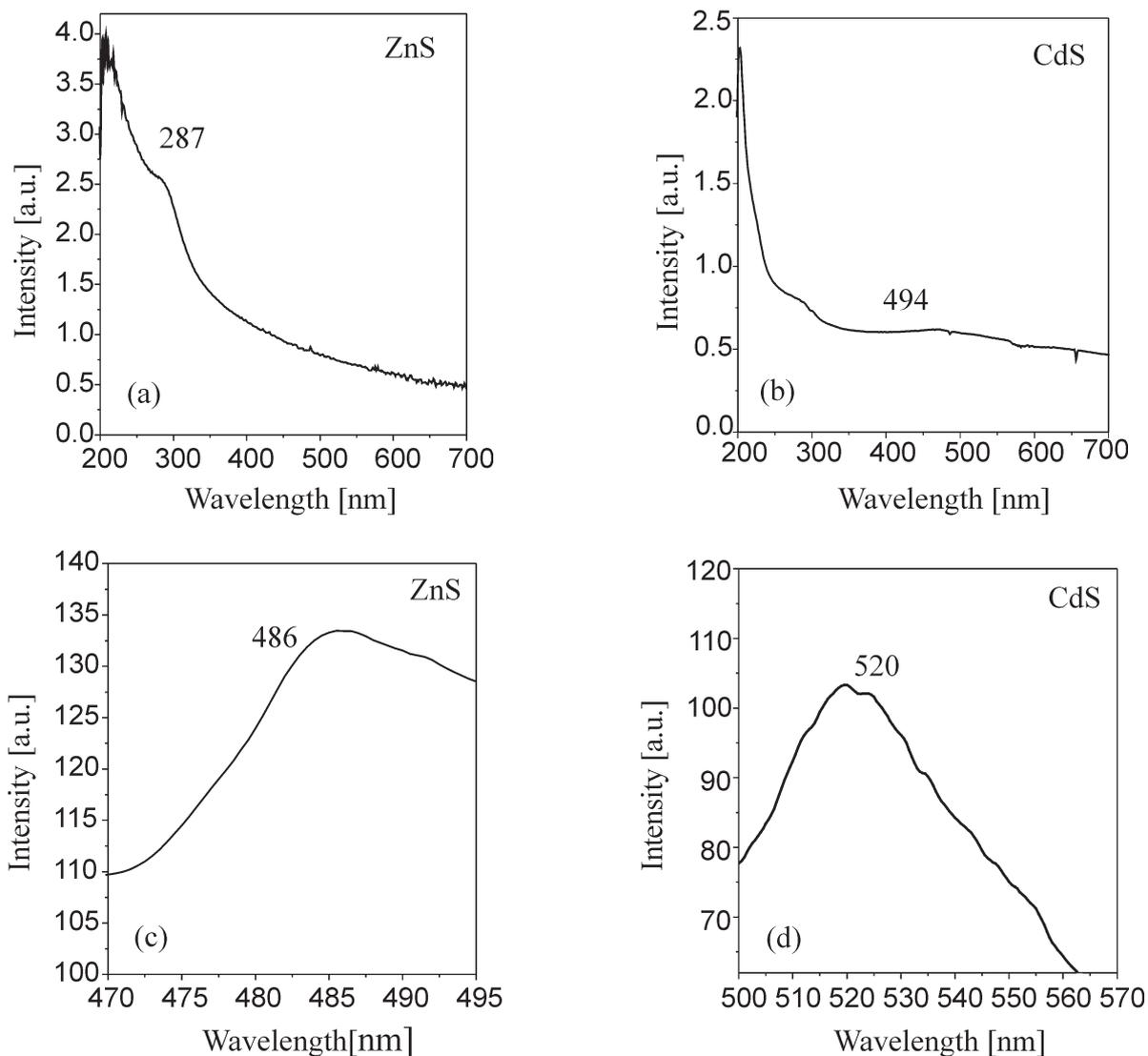
Fig. 3. UV-VIS absorption and PL emission spectra of the products: (a) ZnS – 287, (b) CdS – 494, (c) ZnS – 486, (d) CdS – 520.
