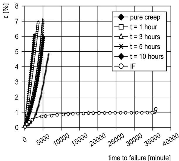
Fig. 3. Strain-time to failure dependences for longer holds.
