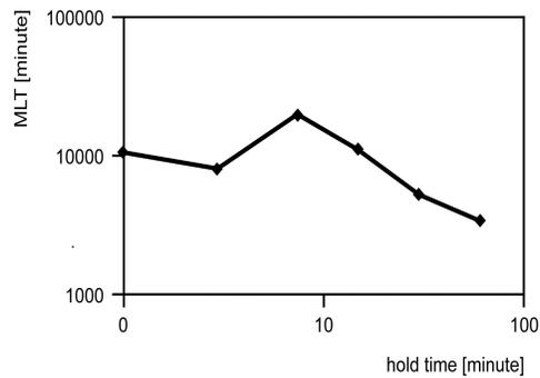
Fig. 5. Plot of the time to failure in terms of the sum of hold time at maximum load.
