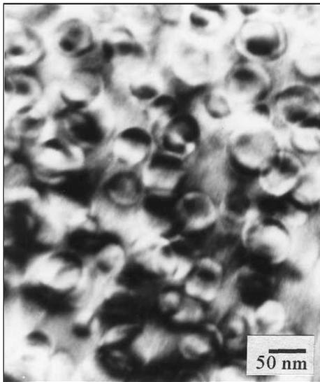
Fig. 1. TEM micrograph of the gamma prime distribution and morphology.
