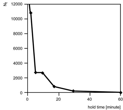
Fig. 6. The dependence of hold time and the number of cycles to failure.
