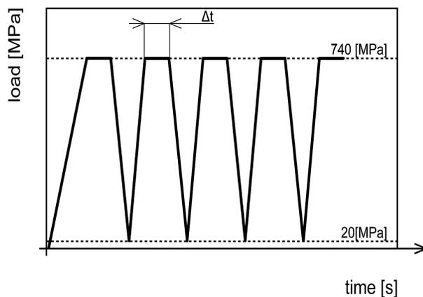
Fig. 2. Diagram of the fatigue loading schedule.
