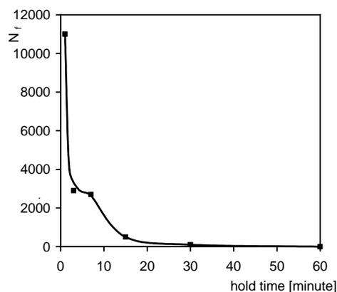
Fig. 9. Model prediction dependence of  $N_f$  as the function of hold time.
