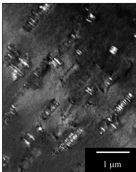
Fig. 4. "Ribbon" like modification of the Mg_{12}Ce stable phase in the as-cast MgCe_3Sc_1Mn_1 alloy in the [0001] direction of the \alpha -Mg matrix.
